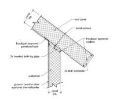
The Insulspan® SIP (Structural Insulating Panel) System is an energy efficient building system that consists of a core of expanded polystyrene (EPS) insulation with oriented strand board (OSB) structurally laminated to the interior and exterior faces. This bulletin provides effective thermal resistance (RSI<sub>eff</sub>/R<sub>eff</sub>) for Insulspan SIP System wall and roof assemblies calculated as per National Building Code of Canada 2010 (NBC 2010), Subsection 9.36.2.
